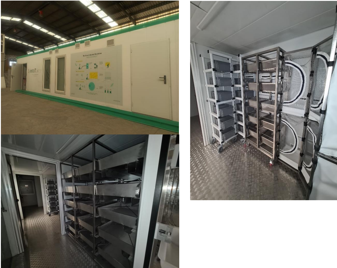
Figure 10. Typology of IPP to be constructed and installed in ISA-CM: Up-left, external view of the container where the walls act as illustration for the project iconography; Down-left, interior part of the container showing fattening area and; Right, breeding ca
